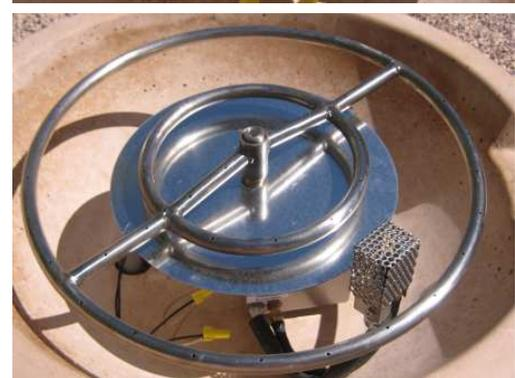
9. Pilot Burner Positioning. Positioning of the Pilot Burner is very important with regards to proper functioning of the AWEIS module. The photo at right shows how the Pilot Burner should be positioned in relation to the fire ring when the install is complete.
